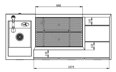
Stainless steel constructionInsulated ice well with dividers<br/>(668x375mm)4 GN 1/9 trays for bar condimentsCustom speedrack for bottlesFour neutral temperature drawers<br/>below for bottlesSink (330xx500mm)Integrated glass rinser in the sinkSliding plastic cutting boardCompartment for organic wasteWaste flap in frontOne drawer for garbage bagRear upstand 20mm at the backDimension (mm): 1500x650x900
